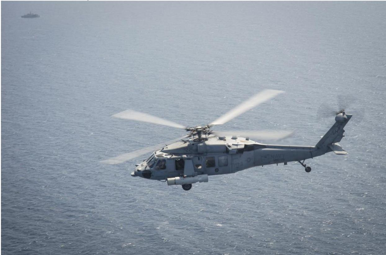
[Seahawk](#) with the standard equipment **nose-mounted** [Raytheon Multi-Spectral Electro-Optical Targeting System \(EOTS\)](#), which also has an [Airborne Laser Mine Detection](#)
