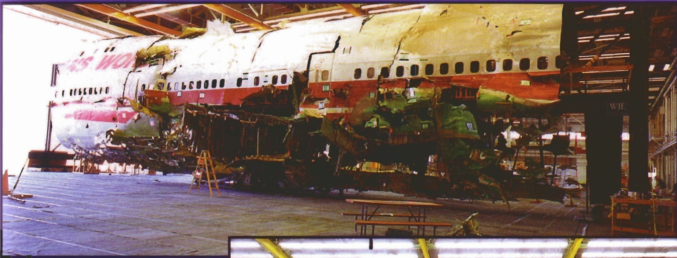
TWA 800 fuselage reconstruction. A photograph taken by the NTSB of the left side of the fuselage. The site of the breach was roughly abeam the L2 door.
